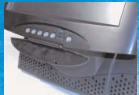
Flip Down Door Protects Liquid Resistant Control Panel
